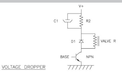
NOTE: The semiconductor can be replaced by a suitable relay.
