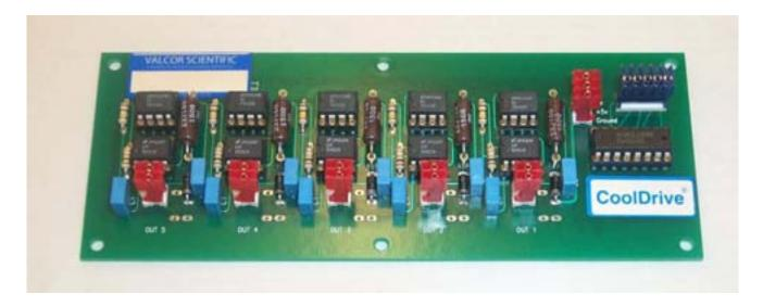
The CoolDrive ® driver circuits by Valcor Scientific, complements Valcor Scientific's SV74, SV75 & SV76 Series of solenoid valves. The CoolDrive ® driver circuit incorporates five drivers on one compact board measuring 6 inches long by 2.3 inches wide. The drive circuit allows for independent operation of five solenoid valves using 5v logic level signals from your PC.
