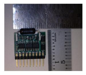
The CoolDrive<sup>®</sup> One Single Valve Driver circuits by Valcor Scientific, complement Valcor Scientific's SV74, SV75 & SV76 Series of solenoid valves. Main applications include valves with extended energized periods, and/or high duty cycle.
